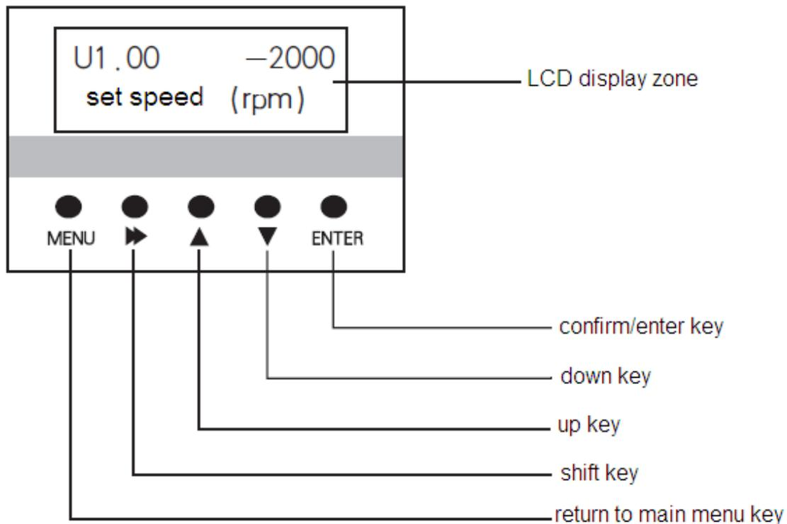
Figure 3-15 PO-S6 Manipulator diagram
