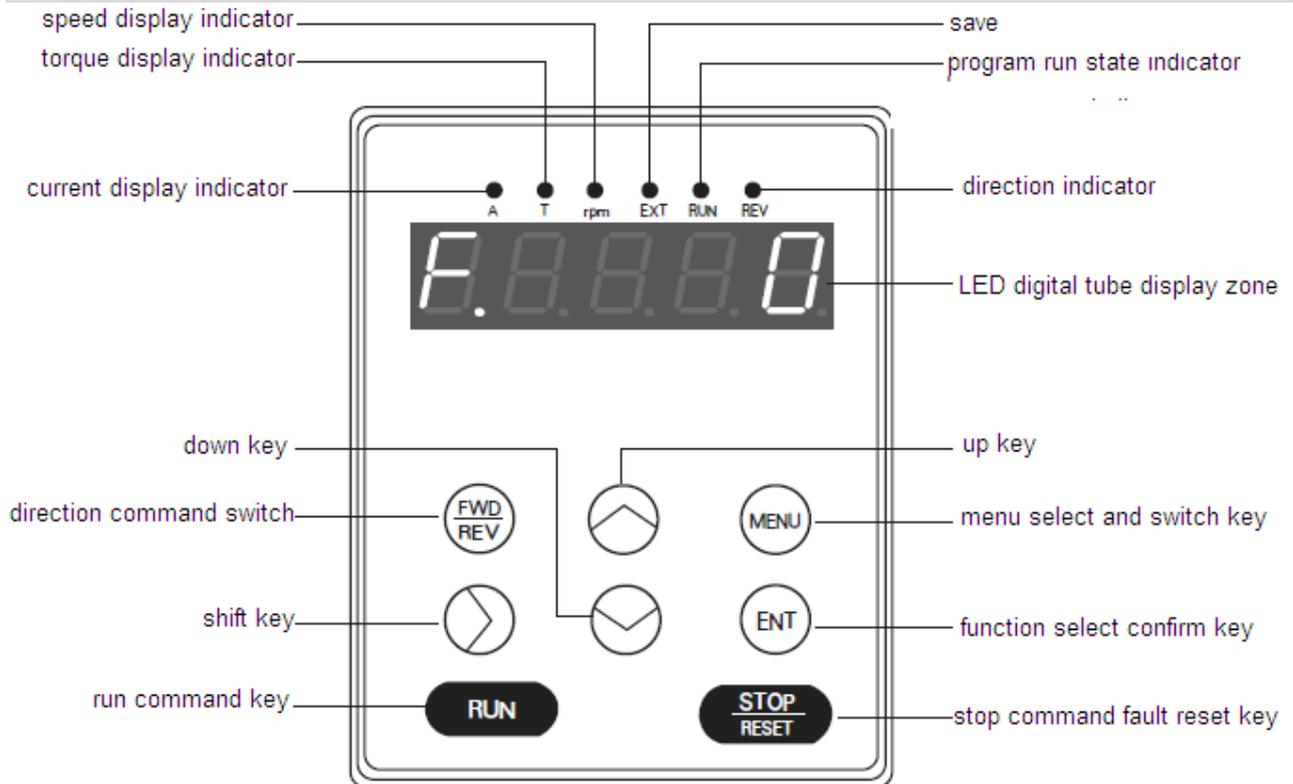
Figure 3-8 Manipulator diagram
