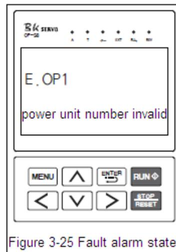
Figure 3-25 Fault alarm state
