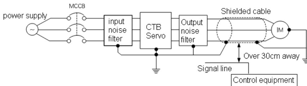
Figure 2-11 Suppress radio interference with output filter
