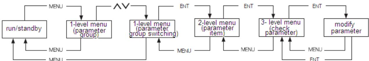
Figure 3-12 3-level menu operation flow chart
