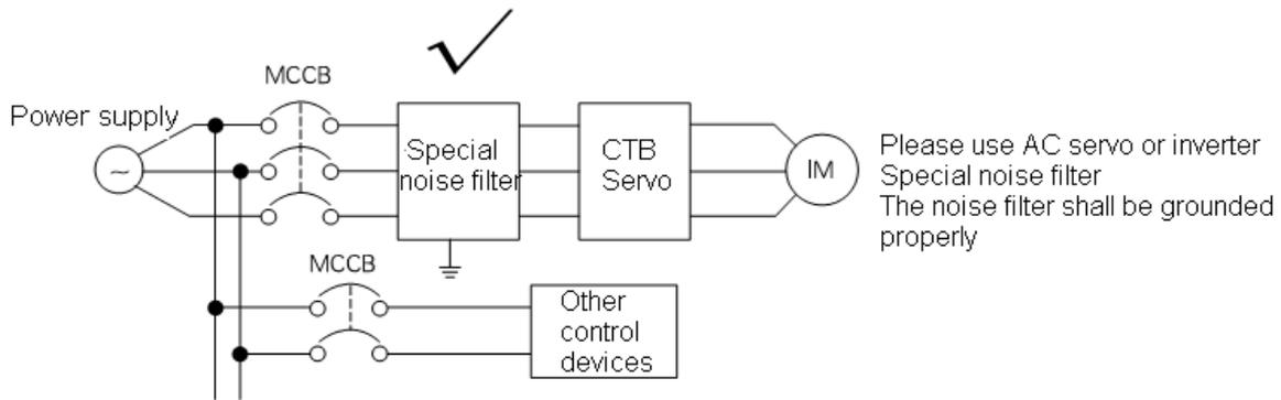
Figure 2-6 Correct installation of noise filter at the input side of the power supply
