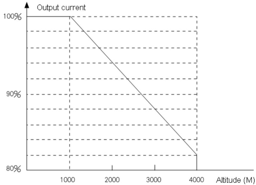
Figure 1-10 Derating curve of rated current of driver and altitude
