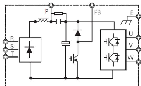
Figure 2-2D 90~160kw main circuit composition
