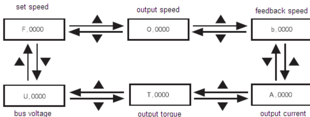
Figure 3-7 Driver operation state monitoring flowchart
