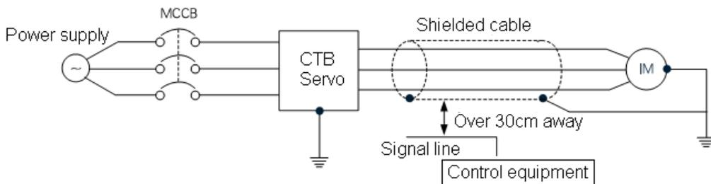
Figure 2-10 Connecting method of shielded cable
