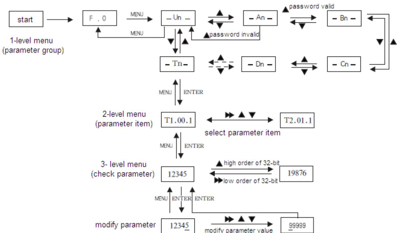
Figure 3-27 2-level menu operation flow chart
