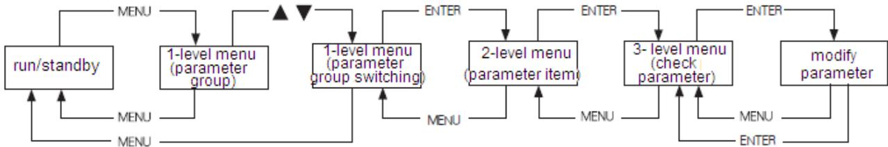
Figure 3-5 3-level menu operation flow chart
