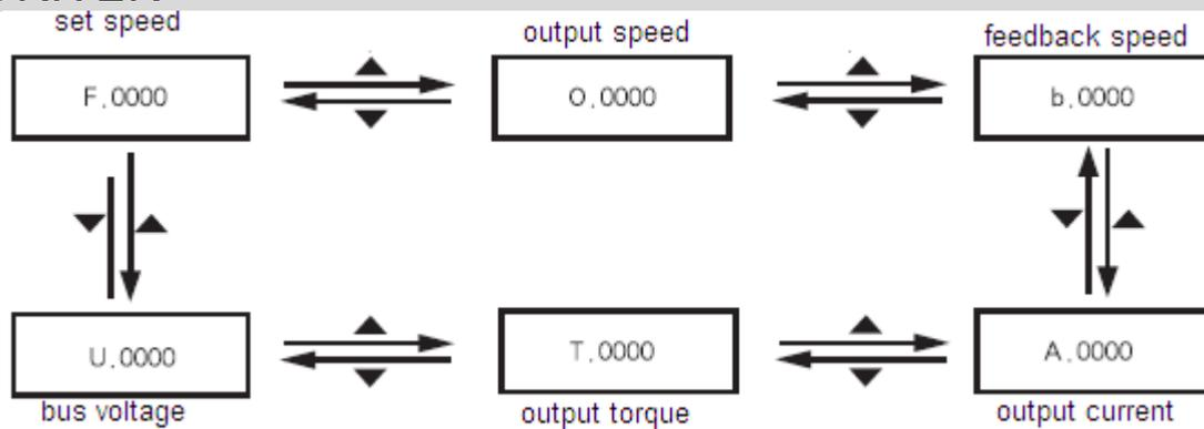
Figure 3-14 Driver operation state monitoring flowchart
