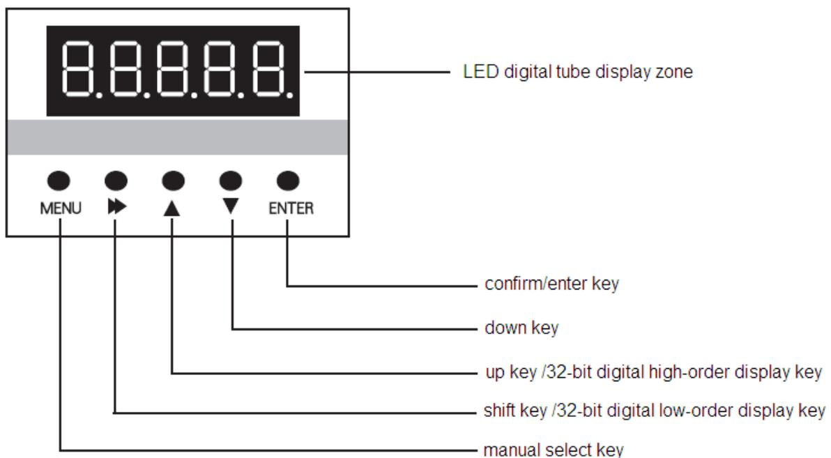
Figure 3-1 Manipulator diagram
