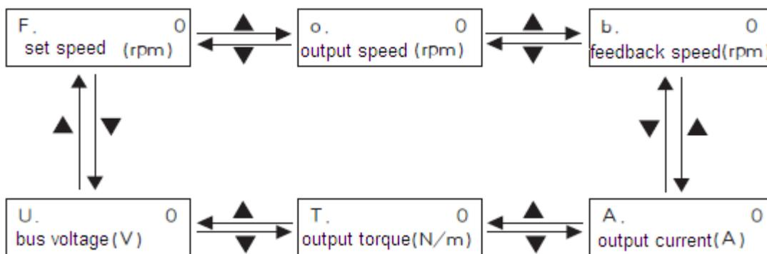
Figure 3-21 Driver operation state monitoring flowchart
