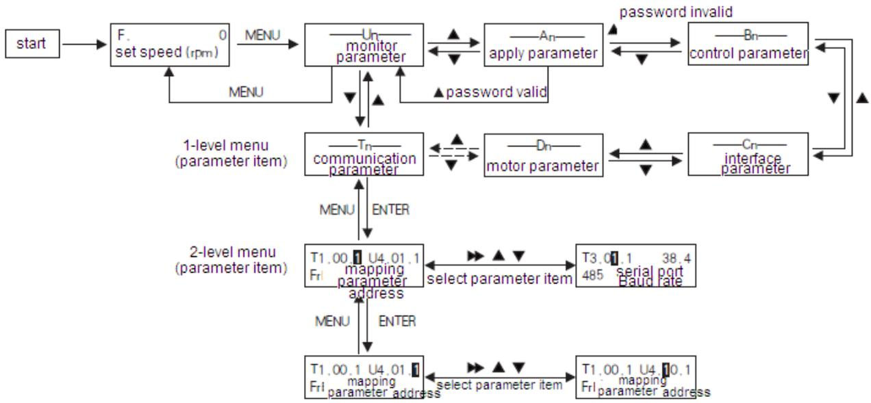
Figure 3-20 2-level menu operation flow chart
