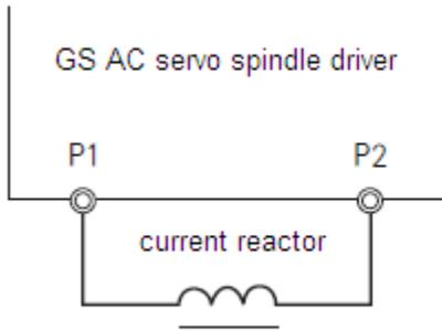
Figure 2-4 DC reactor connection diagram
