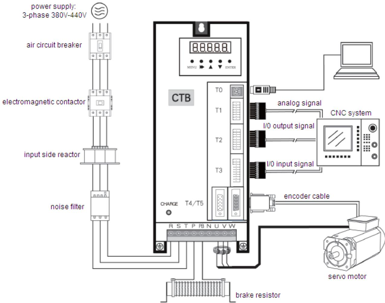
Figure 2-1 Spindle driver and peripheral devices connection diagram
