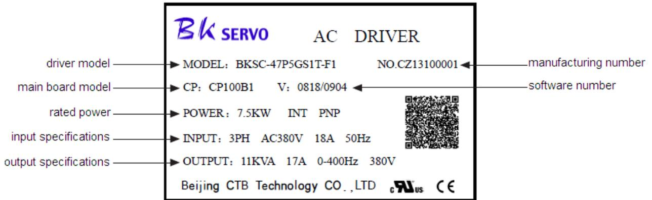
Figure 1-1 AC Servo spindle driver nameplate
