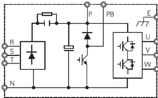
Figure 2-2A 1.5~11kw main circuit composition
