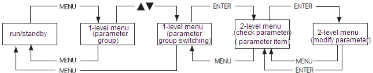
Figure 3-19 2-level menu operation flow chart
