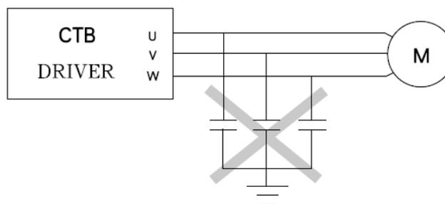
Figure 1-9 Capacitor is prohibited at the output end of controller
