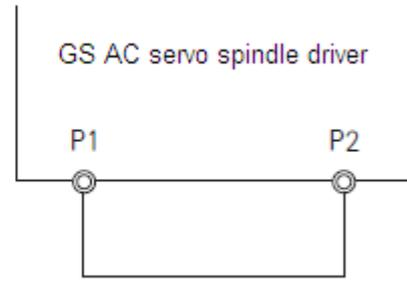
Figure 2-5 Connection diagram without DC reactor
