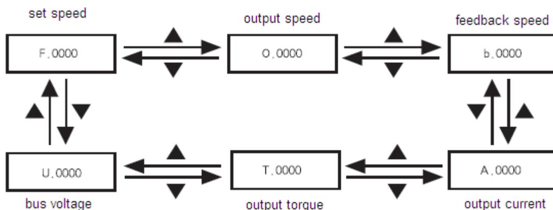
Figure 3-7 Driver operation state monitoring flowchart
