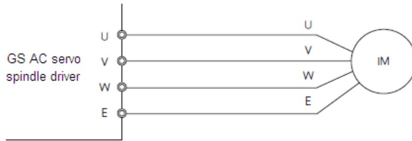
Figure 2-8 Output side wiring
