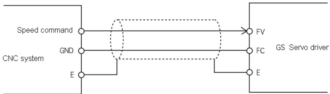
Figure 2-16 Bipolar speed setting is conducted by CNC system
