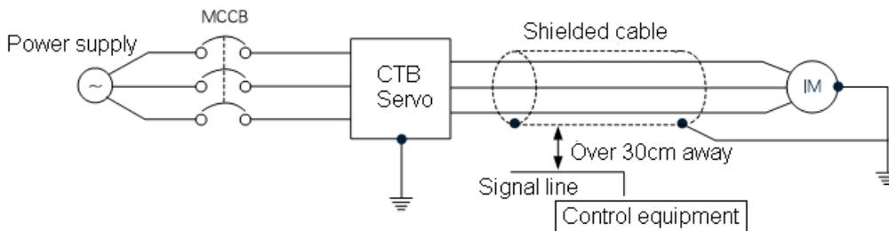
Figure 2-10 Connecting method of shielded cable
