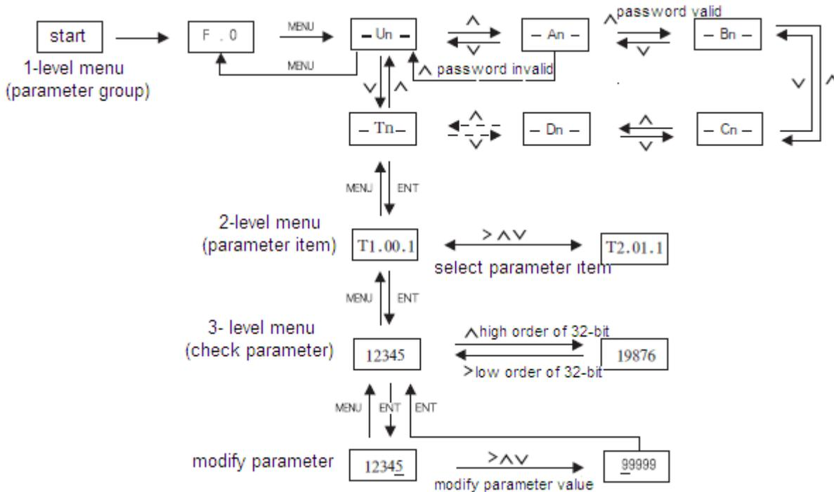
Figure 3-13 3-level menu operation flow chart
