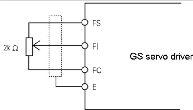
Figure 2-15 Conduct speed setting with internal power
