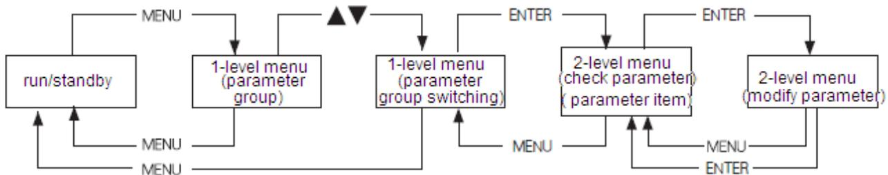
Figure 3-19 2-level menu operation flow chart
