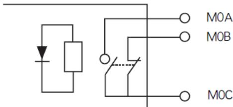
Fault relay output schematic diagram
