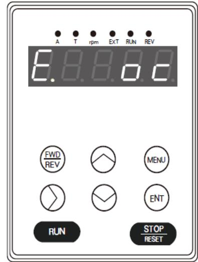
Figure 3-11 Fault alarm state
