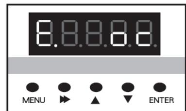
Figure 3-4 Fault alarm state
