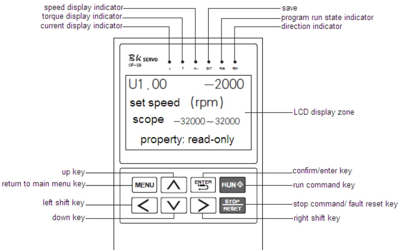
Figure 3-22 PO-S8 Manipulator diagram
