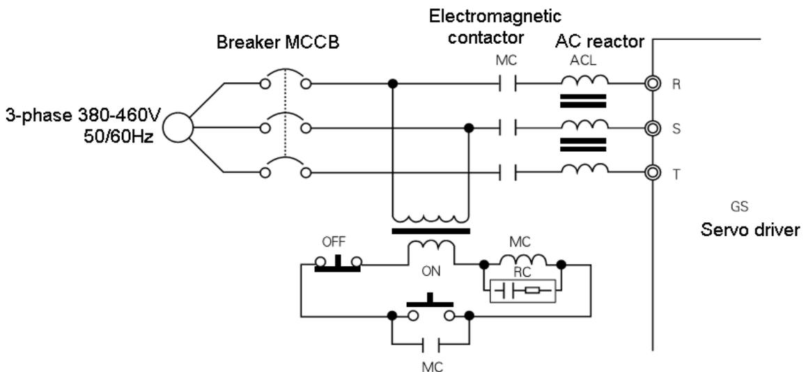
Figure 2-3 Standard wiring diagram for incoming line
