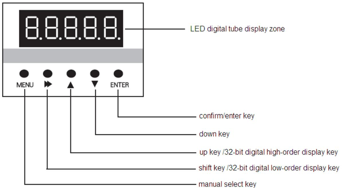
Figure 3-1 Manipulator diagram
