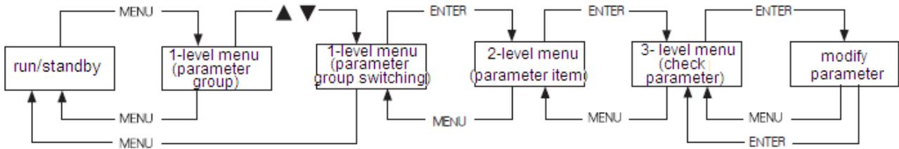
Figure 3-6 2-level menu operation flow chart
