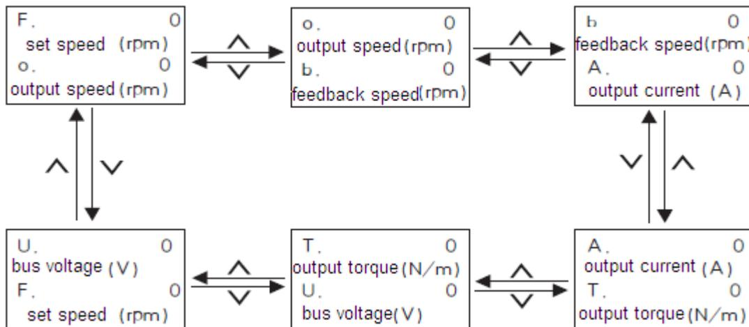
Figure 3-28 Driver operation state monitoring flowchart
