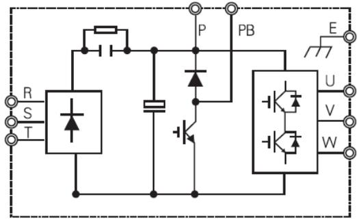
Figure 2-2B 15~30kw main circuit composition
