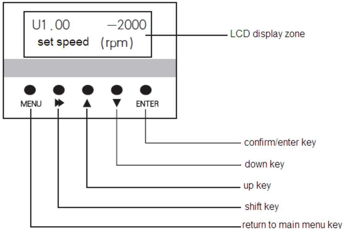
Figure 3-15 PO-S6 Manipulator diagram
