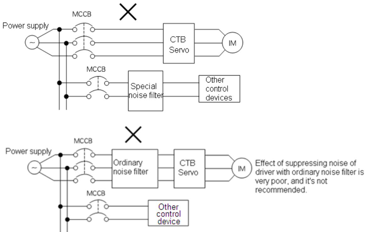
Figure 2-7 Incorrect settings and connection of noise filter at the input side of the power supply
