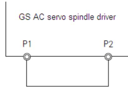
Figure 2-5 Connection diagram without DC reactor
