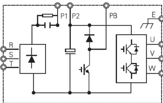
Figure 2-2C 37~75kw main circuit composition
