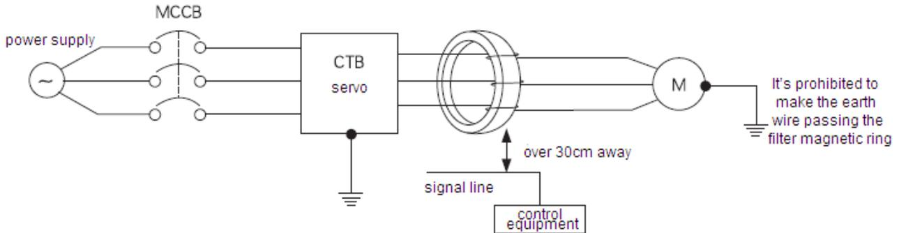
Figure 2-9 Filtering magnetic ring installation diagram
