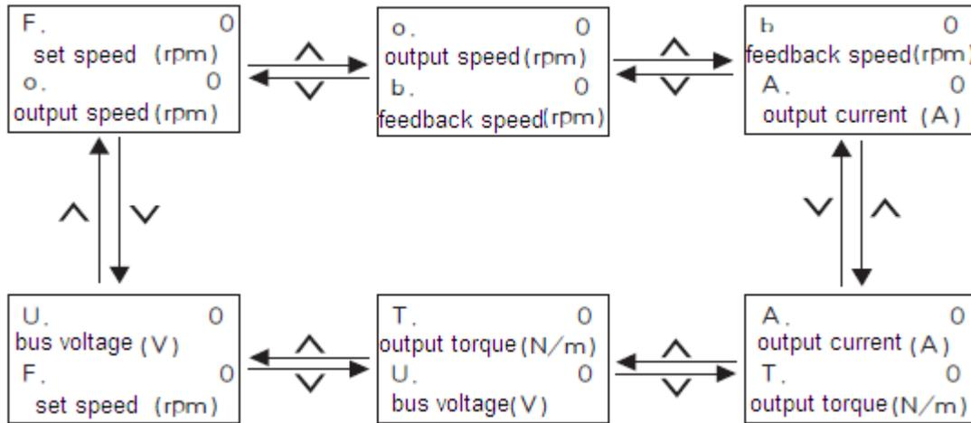
Figure 3-28 Driver operation state monitoring flowchart
